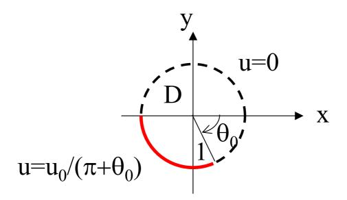
Figure 2: Setup for hot spot problem on circle.
