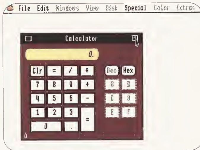
Figure 4. System 6 puts a colorful four-function calculator desk accessory at your fingertips. Click on zoom box for hexadecimal conversions.
